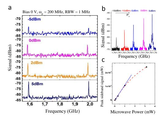
**Figure 4** a) Spectrum analyzer signals with no applied bias, for four different injected powers. The heterodyne signal is no more visible, and two sidebands, generated from the modulation, are present at  $\pm 200$  MHz from 1.8 GHz. b) Sideband signal at increasing injected power from -18 dBm to 5 dBm. c) Sideband peak signal amplitude as a function of the injected microwave power in linear scale. The blue line is the linear fit, whereas the red dashed line is the fit considering saturation.
