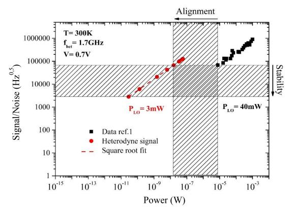
**Fig. 2** log-log plot of the signal-to-noise ratio as function of the QCL power. The noise of the QWIP is calculated using the measured gain and dark current values at room temperature. Black points are data from [17], while red points are the current measurements. The improvement was possible in the horizontal scale thanks to a greater responsivity, in the vertical scale to a better stability.
