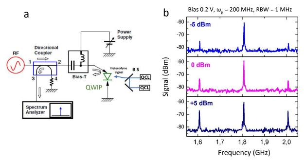
**Figure 3** a) Schematic of the microwave modulation experiment, where the heterodyne signal produced by the two DFB lasers is modulated by a microwave source and biased through a bias T. The signal is recorded by a spectrum analyzer. b) Spectrum analyzer signals with an applied bias of V = 0.2 V, for three different injected powers. The heterodyne signal has a frequency of 1.8 GHz, and two sidebands, generated from the modulation, are distant  $\pm 200 MHz$  from it.
