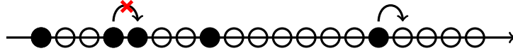
FIGURE 1. A forbidden jump (on the left) and a jump (on the right) in TASEP.
