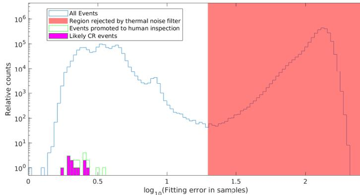
Figure 2: Histogram of time-of-arrival residuals from the direction of arrival fitting. The median residual was time-variable, but typically  $3 \sim 4$  samples. High fitting residuals (chosen to be  $> 12$  times the median residual) usually indicate a spurious trigger caused by random thermal noise—alongside other basic instrumental checks, this is the first cut performed outside the FPGA.
