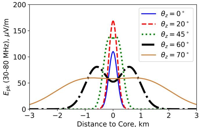
Figure 22: Examples of cosmic ray air shower peak electric fields in the 30 - 80 MHz band as a function of distance from core. These beam patterns are for a  $10^{17}$  eV proton air shower with  $X_{\max}$  corresponding to that energy and zenith angle  $\theta_z$ , observed at the OVRO-LWA altitude of 1.2 km.
