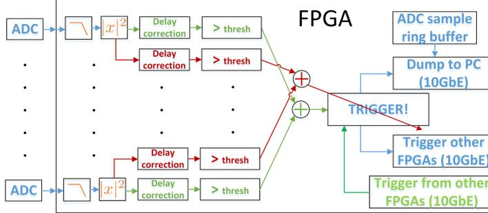
Figure 4: Simplified block diagram of the FPGA system. Full details described in Section 5.
