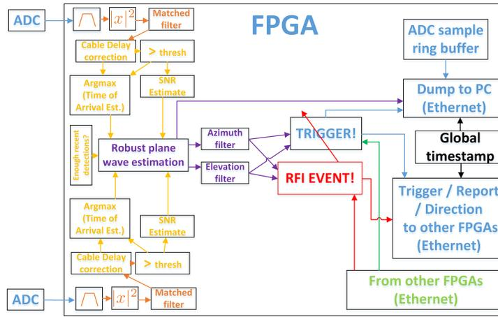
Figure C.33: Block diagram of a proposed, lower bandwidth FPGA firmware. In prototypes, robust planar fitting vastly outperforms the RFI filtering used in Section 5.
