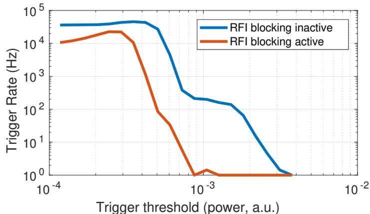
Figure 6: **Top:** event rates both with and without on-chip filtering applied. Each data point was collected at a distinct time in a time-variable RFI environment, which limits interpretability of the data. Because each data point is taken at a distinct time, it is not possible to differentiate between time variable RFI and random thermal noise using the data from this plot.
