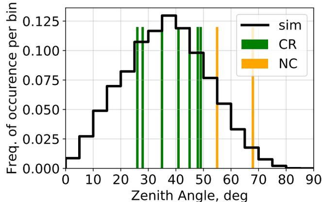
Figure 28: Frequency of occurrence of cosmic rays that trigger the OVRO-LWA detector ( $\text{SNR}_a > 5.7$ ) and analysis cuts. The zenith angles of cosmic ray candidates (CR) are shown in green bars with the “no call” (NC) events shown in orange bars.
