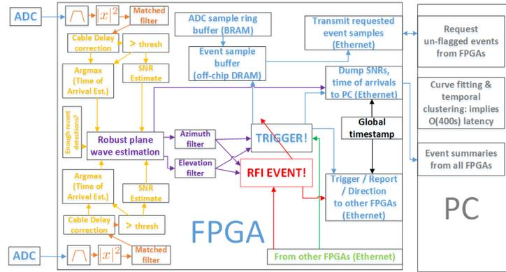
Figure C.35: Block diagram of a proposed, lower bandwidth FPGA firmware, with the use of an additional PC co-processor to further reduce bandwidth by avoiding the transmission of airplane-driven or temporally clustered events.
