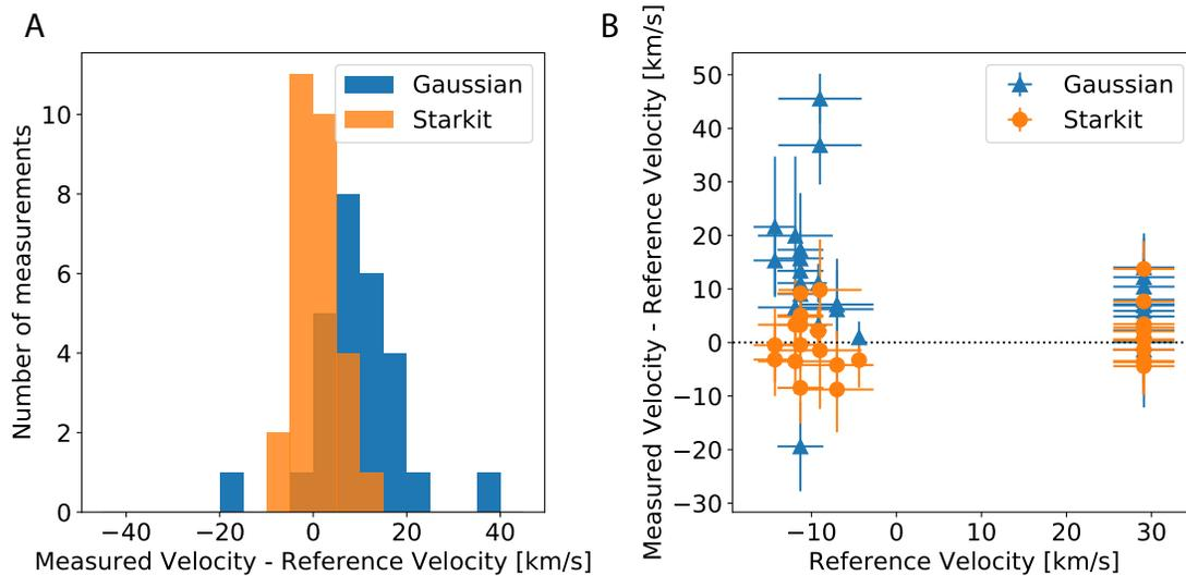
Figure S3: **A:** Histogram of the differences between radial velocity measurements and reference values of standard stars given in Table S3. **B:** Differences between radial velocity measurements and reference values compared to their reference velocity for each individual measurement.
