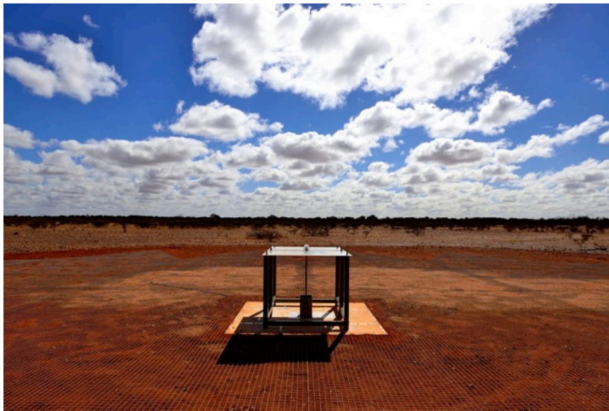
Figure 6-1 An EDGES antenna.
