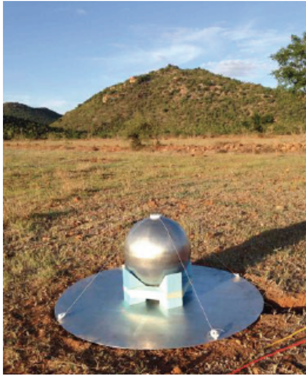
Figure 6-3 SARAS-2 Sphere-disc antenna
