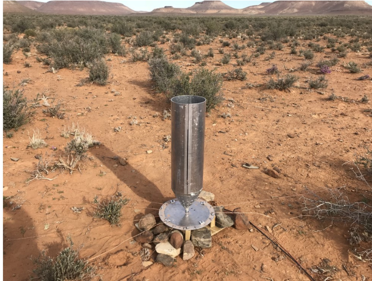
Figure 6-5 The 84 cm antenna deployed at Karoo Site 4 in July 2018. Ground radial wires attach the center plate. The calibration system and LNA are mounted in the RF box below this plate.
