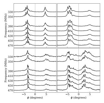
**Figure 2.** Profiles of four example single pulses used in the analysis with the seven frequency channels plotted vertically with the highest frequency at the bottom. The pulses have been dedispersed and aligned with respect to the defined fiducial plane (at phase  $\phi = 0^{\circ}$ ) as described in the text.
