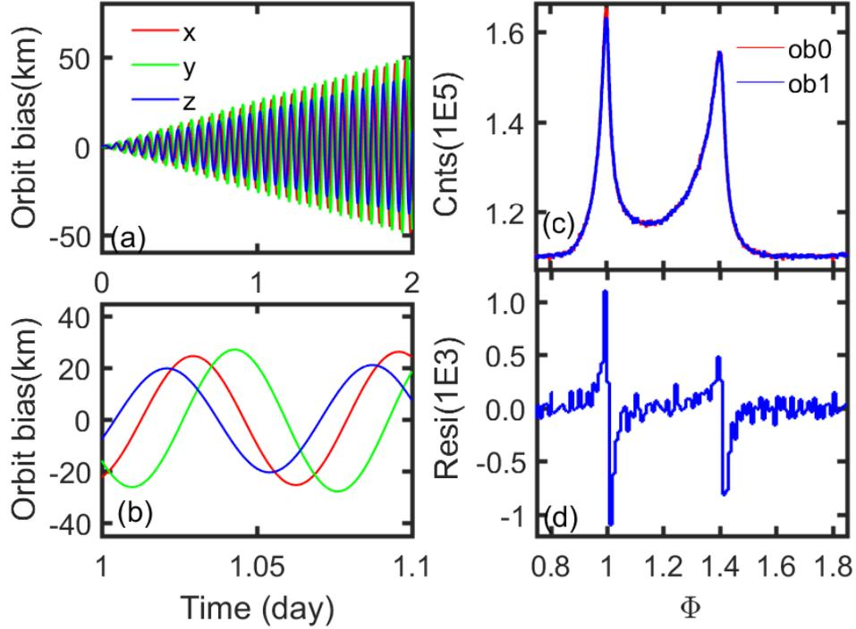
Fig. 1.— The orbit deviation due to the change of initial orbit element ‘semi-major axis’ by 200 m and its effects on the profile. (a) orbit deviations for 2 days; (b) zoom in of the orbit deviations. (c) distortion of pulse profile induced by the change of initial element. The red line represents the ‘standard’ profile generated with ‘ob0’, and the blue one represents the distorted profile generated with ‘ob1’; (d) differences between the ‘standard’ profile and distorted profile
