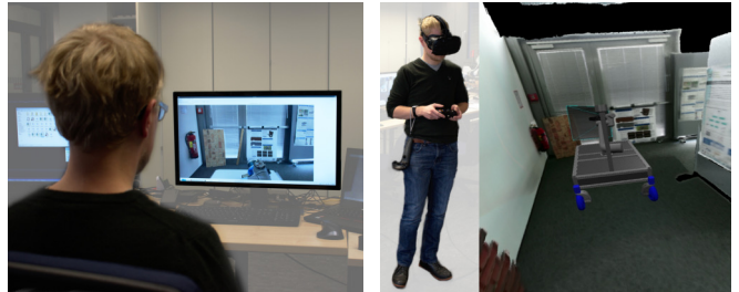
Fig. 5. Teleoperation experiment. Left: Baseline experiment with wide-angle camera feed. Right: Teleoperation using the proposed VR system.
