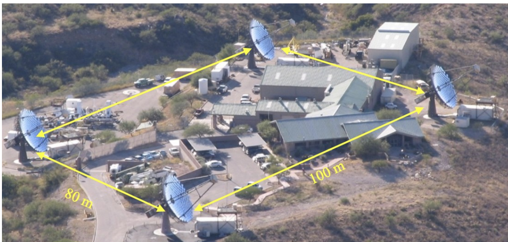
Figure 1: Aerial picture of the VERITAS 4 telescope Imaging Air Cherenkov Telescope Observatory, including approximate telescope baseline separation distances
