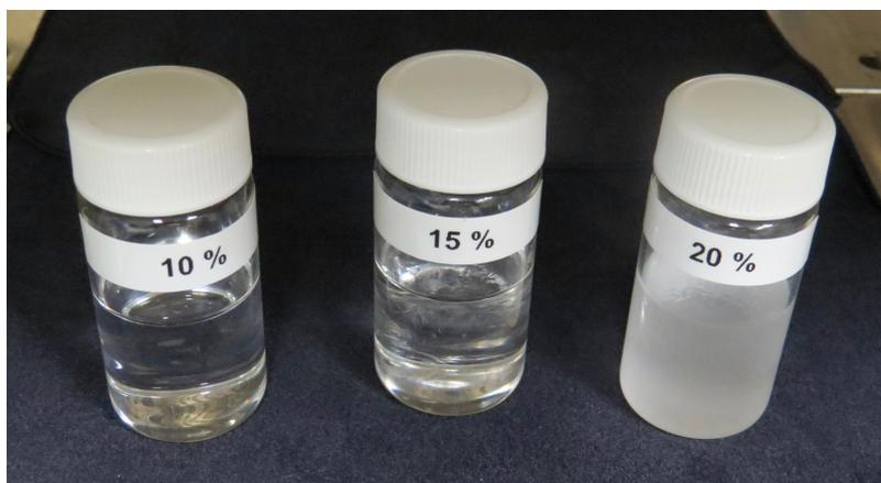
**Figure 5.** The picture shows three samples with 10% (left vial), 15% (middle vial) and 20% (right vial) of paraffin wax at 30°C. The scintillator was cooled from above 40°C at a cooling rate of about 2 K/hour and kept overnight at 30°C. The outer diameter of the vials is 2.8 cm. At 25°C all the samples are opaque.
