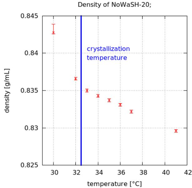
**Figure 6.** The plot shows the temperature dependence of the scintillator density. The series of measurements started at 41°C and then the scintillator was slowly cooled down. The error bars indicate the estimated uncorrelated uncertainty between data points. An extra systematic uncertainty contribution was added to the upper bar at 30°C to account for the possible effects of gas bubbles, as described in the text.
