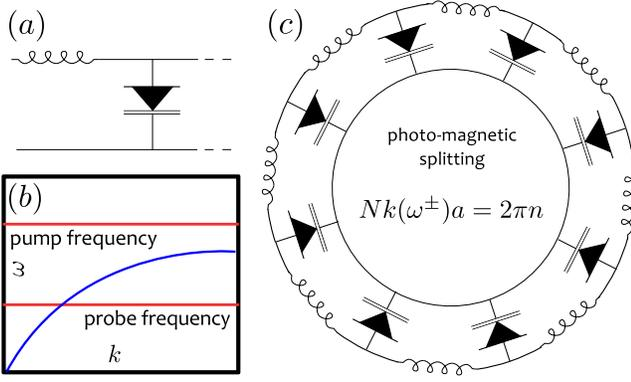
FIG. 5. (a) The capacitor in a conventional transmission line is replaced by a varactor, whose capacitance varies with the voltage across it. The inductors are also assumed to vary with the bias current. (b): Schematic dispersion showing the pump and probe frequencies. (c) Discrete elements combined into a loop to demonstrate the presence of a photo-magnetic field.
