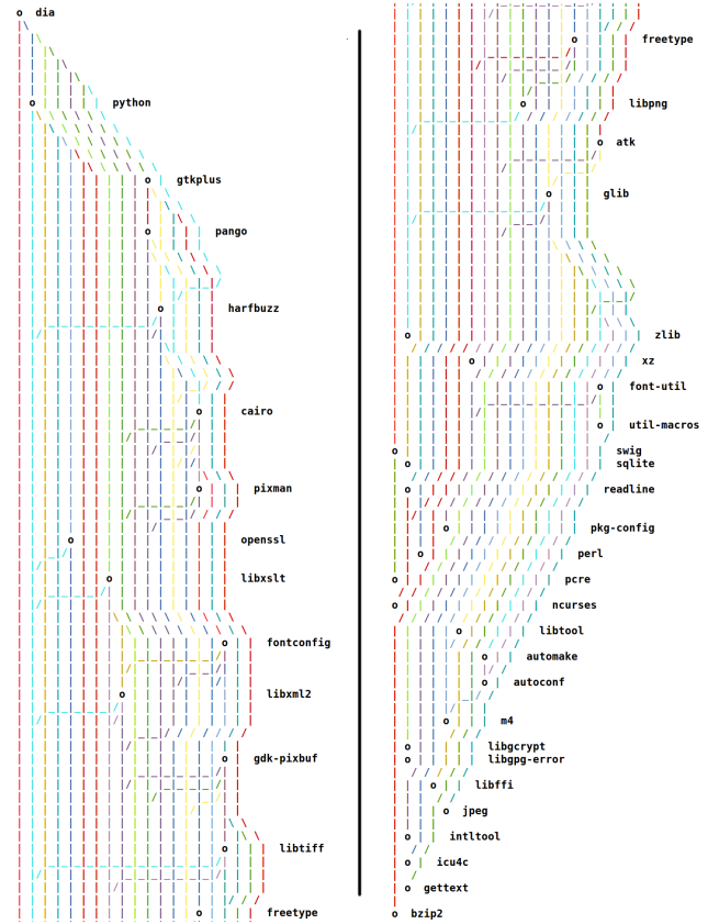
Fig. 6: git-style package dependency graph of dia (also shown in Fig. 1). The freetype node has been duplicated to show alignment between the two halves.
