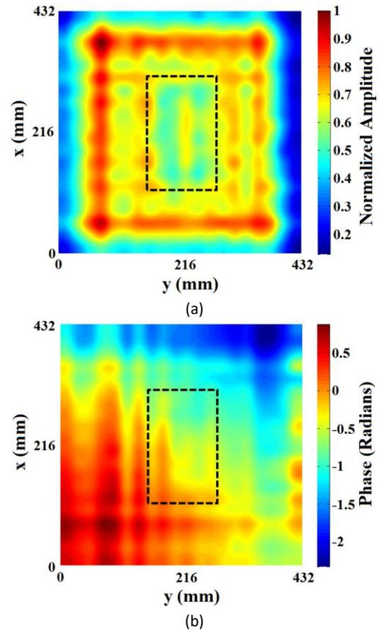
Fig. 15 Reconstructed back-propagated through-the-wall images of the concealed dielectric box at the object plane,  $z=18$  cm (a) reconstructed amplitude (b) reconstructed phase.
