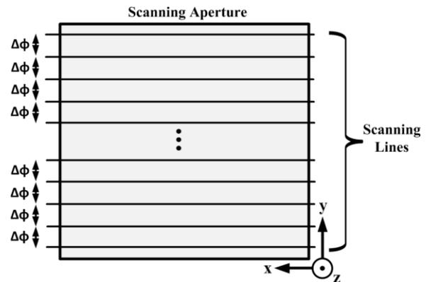
Fig. 2 Linear phase shift in the y-axis.
