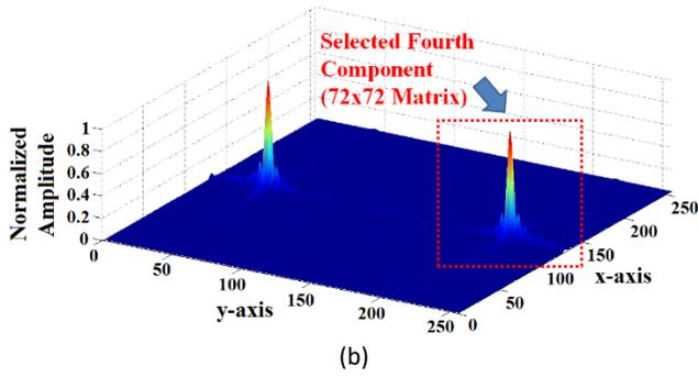
Fig. 13 PWS of the concealed dielectric box after the average value of the intensity matrix was subtracted prior to being Fourier transformed (a) along the y-axis (b) three-dimensional.
