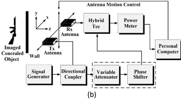
Fig. 1 Indirect microwave holographic TWI system (a) measurement set-up (b) diagrammatic representation.
