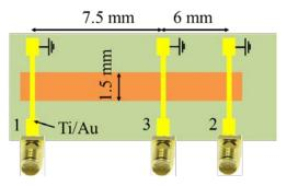
Fig.1. Schematic view of the YIG waveguide with three antennae.
