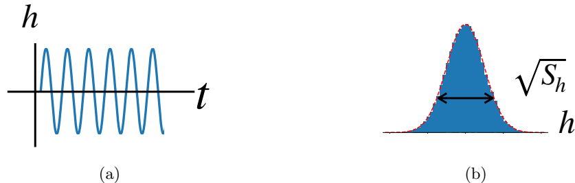
Figure 25: Different signal priors for h(t) . Panel (a): Deterministic (sinusoid) signal prior. Panel (b): Stochastic signal prior. For the stochastic signal prior, h(t) values are drawn from a Gaussian distribution with variance S_h .
