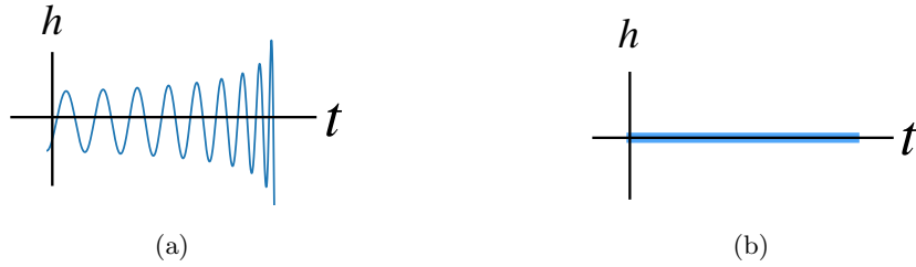
Figure 26: The two components of the mixture signal prior for the Bayesian BBH merger search. Panel (a): With probability \xi , the signal prior for h(t) is a chirp waveform. Panel (b): With probability (1 - \xi) , the signal prior for h(t) is just noise, i.e., h(t) = 0 .
