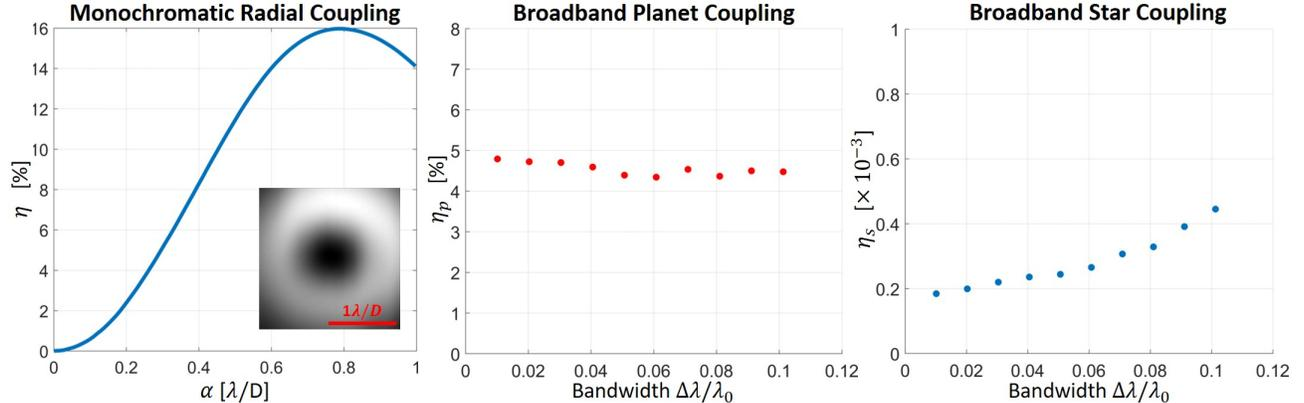
Figure 3: (left) Azimuthally averaged radial coupling,  $\eta$ , with 635 nm laser light and a charge 1, monochromatic vortex mask. The inset is the two dimensional coupling map. (middle) Azimuthally averaged peak planet coupling,  $\eta_p$ , in broadband light at various bandwidths centered around  $\lambda_0 = 790$  nm and with a charge 2 polychromatic vortex mask. (right) Same as middle, but showing the null depth or “stellar coupling”,  $\eta_s$ .
