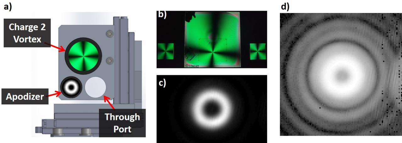
Figure 5: (a) Model of the pupil mask stage for KPIC. (b) Charge 2  $K$ -band vector vortex masks being considered for deployment in KPIC as viewed in cross-polarization. (c) The PSF produced by the vortex masks in (b) when placed in a pupil plane, which takes on the expected donut shape. (d) Same as (c), but on a logarithmic scale.
