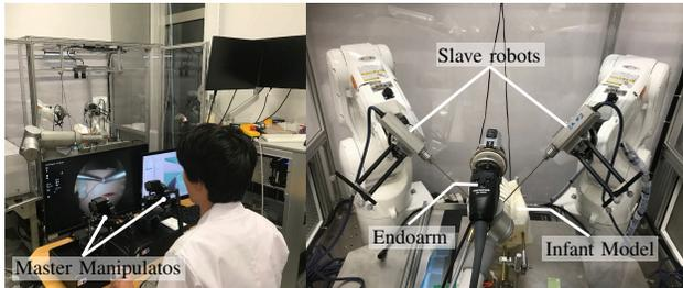
Fig. 6. Master-slave robotic system. Master-side (left), slave-side (right).
