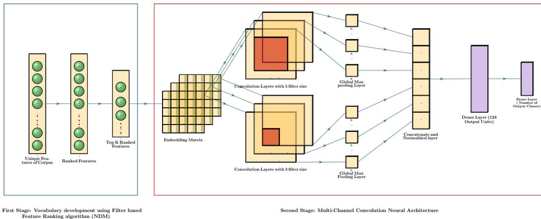
Fig. 1: Proposed Two Stage Classification Methodology
