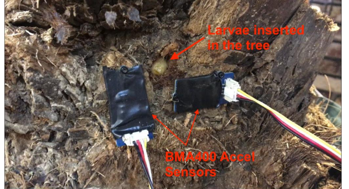
Fig. 20: Position of the sensors to detect Red Palm Weevil (Outside Sensors)
