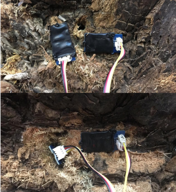
Fig. 19: Sensor Placement on the Palm Tree. The bottom figure corresponds to first scenario with one sensor inside and one sensor outside. The top figure corresponds to the second scenario with two sensors outside
