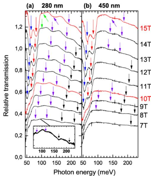
**FIG 1.** Magneto-optical spectra in the mid-infrared for magnetic fields between 7 T and 15 T measured in a 280 nm **(a)** and a 450 nm **(b)** Cd<sub>3</sub>As<sub>2</sub> epilayer. Transmission minima are marked by colored arrows: blue and red denote two cyclotron resonance transitions, purple and black denote two series of interband transitions, and green stands for the combined resonance. The inset in (a) is a vertical zoom (x3) of the 7 T spectrum.
