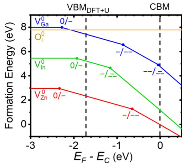
**Figure 5.** Formation energy versus Fermi level for gallium, indium, and zinc vacancy and oxygen self-interstitial acceptor-like defects using the DFT+U band gap for *a*-IGZO under oxygen-poor conditions.
