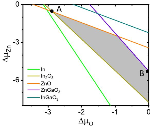
**Figure S2:** Chemical potentials with respect to the  $\Delta\mu_{Zn} - \Delta\mu_O$  phase space. The stability window is shaded in gray. Points A and B correspond to O-poor and O-rich chemical potentials, respectively.
