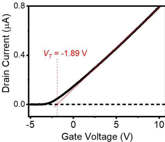
$I_D - V_G$  transfer curves from device measured shown in Figure 1 shows a threshold voltage of  $V_T \sim -1.89$  V in Fig. S1, corresponding to the value predicted for our experimentally measured deep acceptor trap density (see Fig. 1c, red dashed line).
