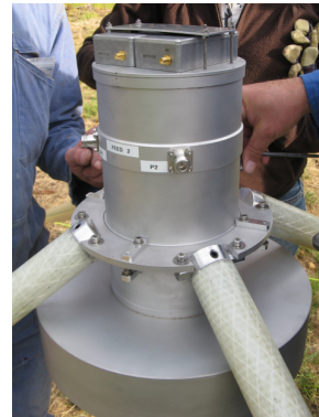
Figure 3. Photograph of a feed: The two amplifiers for H and V probes are located in the two boxes at the top.
