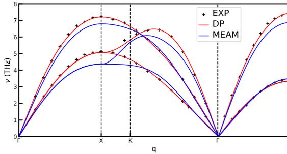
FIG. 5: The DP and MEAM results of phonon dispersion relations for Cu are calculated by phonopy [38] and its LAMMPS interface phonolammps [39] at  $T = 49$  K with the supercell size being  $10 \times 10 \times 10$ . Here  $q$  denotes the wave number and  $\nu$  the frequency. The experimental data are taken from Ref.[40].
