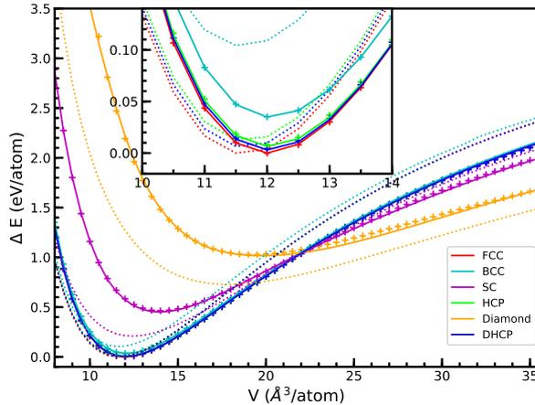
FIG. 4: EOS curves for Cu. Solid lines, dotted lines, and plus markers denote DP, MEAM, and DFT results, respectively. The energies of MEAM are shifted so that the MEAM energy of a stable fcc structure equals that given by DFT. DFT based relaxations fail for some hcp structures with volume per atom larger than  $30 \text{ \AA}^3$ . Therefore, the corresponding DFT predictions are not shown. The diamond, sc, and dhcp structures are not explicitly included in the training data of the DP model.
