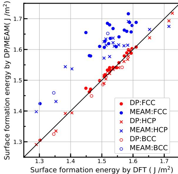
FIG. 6: Surface formation energies for fcc, hcp and bcc-lattices of Cu. All the nonequivalent surfaces with Miller index values smaller than 4 are taken into the consideration for the fcc lattice. For the hcp and bcc lattices, the results for the nonequivalent surfaces with Miller index values smaller than 3 are included.
