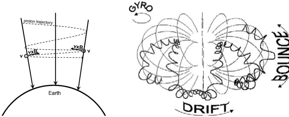
Figure 8.1: (left) Schematic diagram showing the Lorentz force as a particle moves into the magnetic field gradient at Earth's poles. [Fig. II:11.2] (right) Schematic diagram of particle motion in a dipole magnetic field. [Fig. II:11.4]
