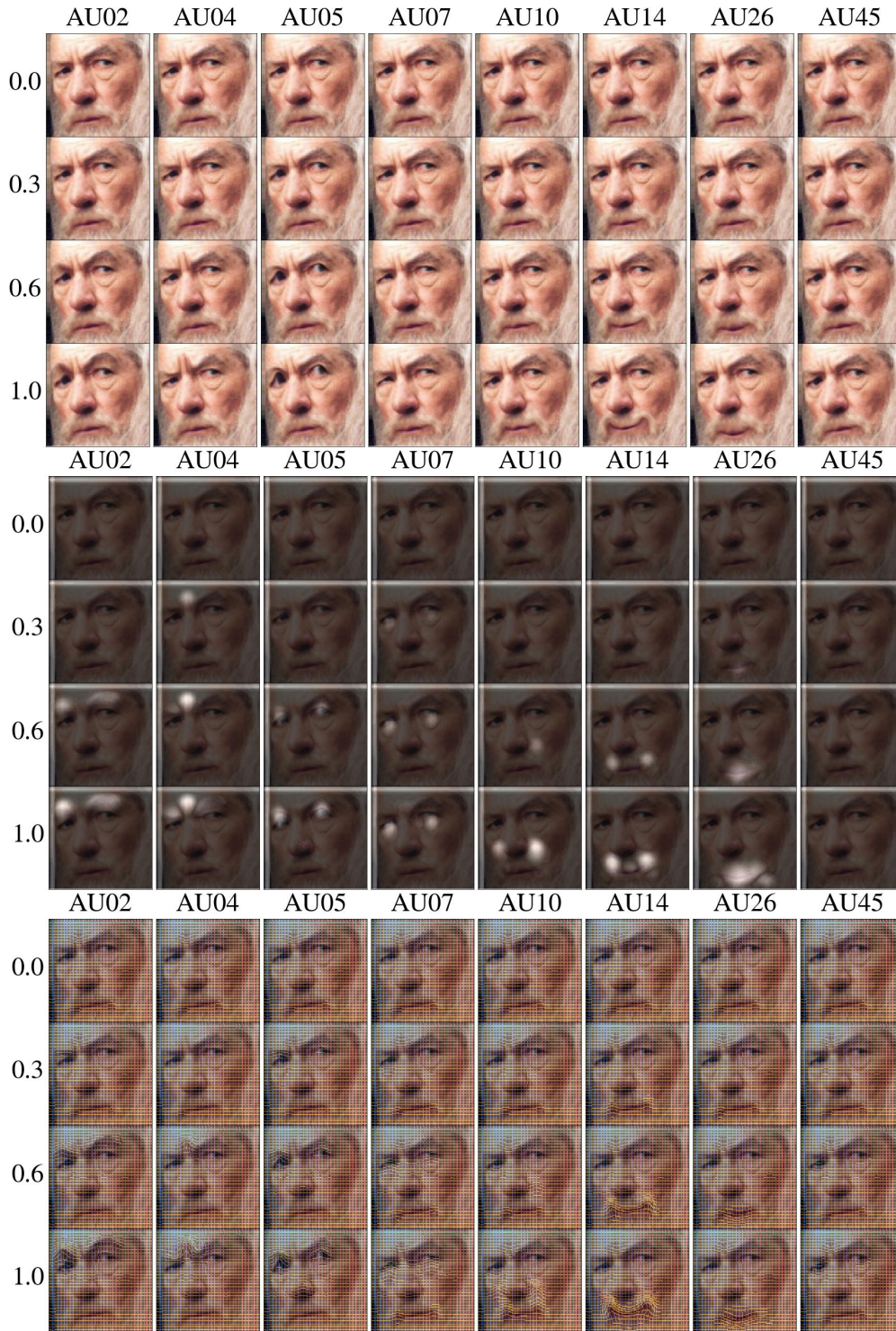
Figure 11: Effects of Single AU editing on the Deformed image \mathcal{I}_y^* . In this figure we show the effects of changing single AU activations on the deformed input image. Top: As can be seen, changing the intensity of AUs causes smooth changes in facial regions. Middle: This figure shows the regions of the face that are deformed as we change the intensity of each AU. We see that the movement is only restricted to regions of the face relevant to the corresponding AU being changed, akin to the results of true facial movement. Bottom: Similar to the figure in the middle, looking at the deformation grid, we see that the movement is only restricted to regions of the face relevant to the corresponding AU being changed.
