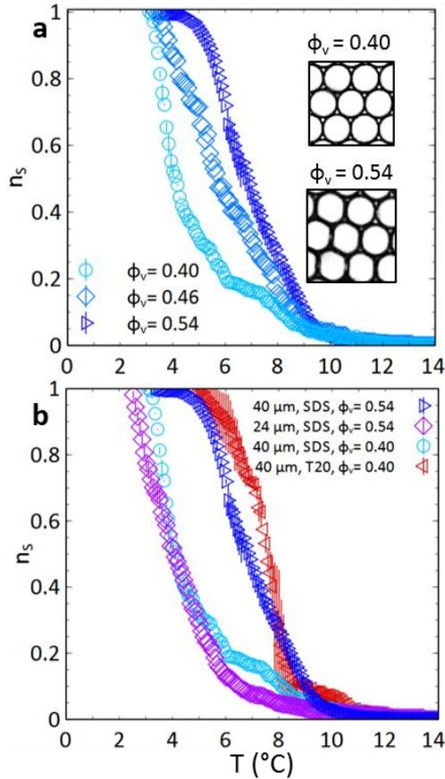
**Fig. 2.** Solid fraction as a function of temperature for (a) SDS-stabilized emulsions at volume fractions of 0.4, 0.46, and 0.54,  $D = 40 \mu\text{m}$  (b) emulsions with droplet sizes of 24 and  $40 \mu\text{m}$  and surfactants of SDS and Tween 20. The insets in (a) show the droplet packing at volume fractions of 0.4 and 0.54. Error bar is standard deviation from two trials.
