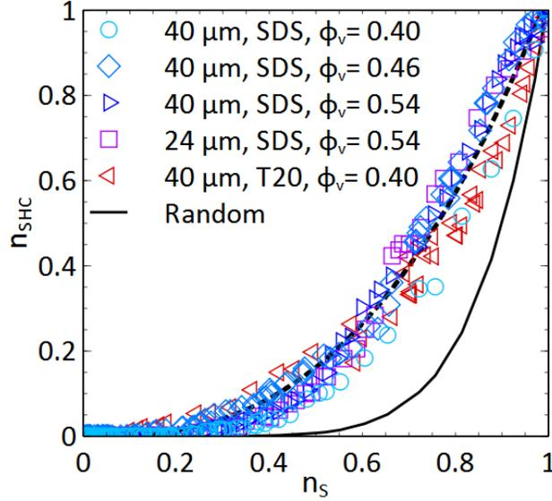
**Fig. 3.** Number density of solid hexagonal clusters as a function of solid fraction for emulsions with different droplet size, surfactant and volume fraction. The dashed and solid lines show the power law fit to the data and prediction from random nucleation simulation respectively.
