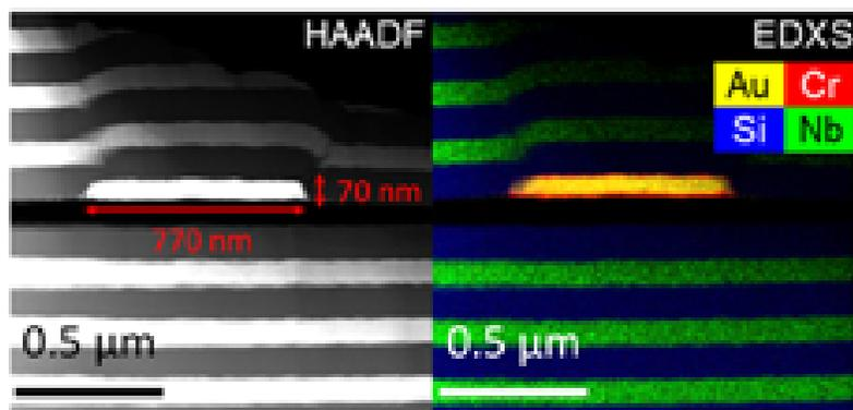
FIG. 6. **HAADF and EDXS** STEM High Angle Annular Dark Field (HAADF) image of the mirror pairs surrounding one gold contact. A map of chemical composition acquired by Energy Dispersive X-ray Spectroscopy (EDXS) is shown on the right.  $\text{SiO}_2$  and  $\text{Nb}_2\text{O}_5$  mirror pairs, shown blue and green respectively, surround the gold contact, yellow, and cavity, shown in black. Scale bar 500 nm.
