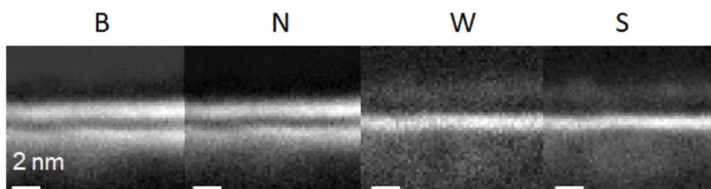
FIG. 7. **EELS of the heterostructure** Electron energy loss spectroscopy (EELS) mapping of hBN encapsulated  $\text{WSe}_2$  monolayer for different elements.
