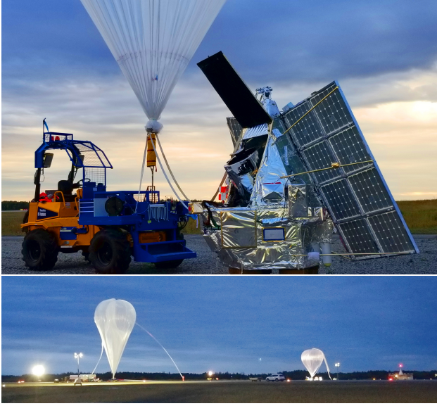
Figure 3. SUPERBIT 2019 pre-launch (site: Timmins, Ontario) secured by a launch support vehicle beneath the tow balloon (top); this smaller tow balloon (bottom, right) provides neutral buoyancy for launch and is secured during primary balloon (bottom, left) inflation.
