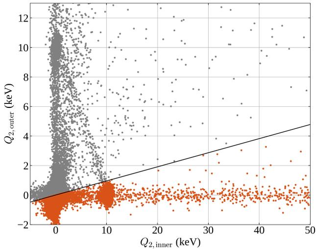
FIG. 4: Signal amplitude in the outer vs. the inner charge channel for side 2 of detector T2Z2 ( $Q_{2,\text{outer}}$  vs  $Q_{2,\text{inner}}$ ). The cut line that removes events with an outer signal above a given fraction of the total signal is shown. At energies below  $E_K$  (10.37 keV) the line cuts into the noise distribution, removing some of the events with a real outer fraction below the threshold. This effect is modelled and accounted for in the final efficiency calculation.
