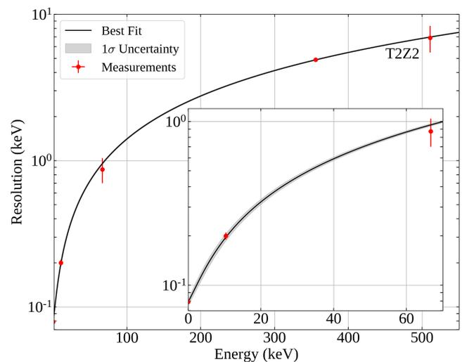
FIG. 7: The fitted resolution model used in the iZIP analysis, for the example of detector T2Z2. The measured peak widths (points) are used to determine the best-fit curve (solid line) and  $1\sigma$  uncertainty band (shaded region). The inset plot shows the same data, zoomed in to the region between 0 and 70 keV.
