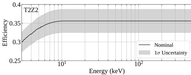
FIG. 6: The efficiency for detector T2Z2 used in the present iZIP analysis. The nominal value (solid line) and  $1\sigma$  uncertainty (shaded region) are shown.
