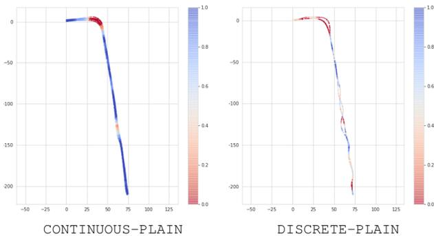
Fig. 6: Qualitative comparison of autonomy between a good model and a lagging one. The graphs show aggregation of few trials (test drives) by these models on the route `factory_city-tunnel-bt10`. The color depicts scale between full autonomy in all trials (blue) and human takeover in all trials (red). Graphs for other models and other routes are available on the project webpage <http://bit.ly/34xh7z4>.
