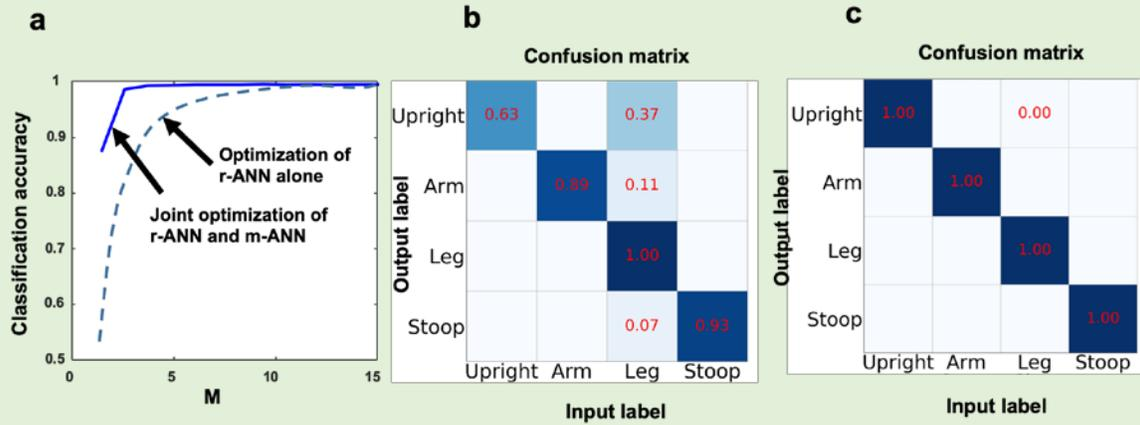
**Figure 4.** Selected experimental results of in-situ gesture recognition directly from a reduced number of measurements. (a) the dependence of the recognition accuracy on the number of coding patterns of the programmable metasurface. (b) The classification confusion matrix with the optimization of the r-ANN alone, where  $M=3$ . (c) The classification confusion matrix with the joint optimization of the r-ANN and m-ANN, where  $M=3$ .
