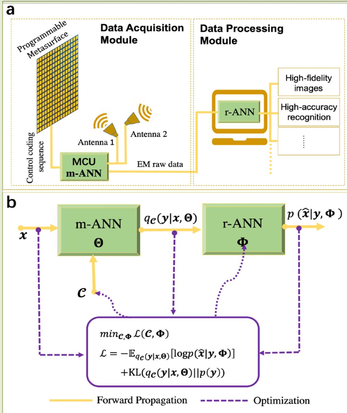
**Figure 1. Working principle of the intelligent sensing system.** (a) The intelligent sensing system consists of two data-driven learnable modules, i.e., the m-ANN-driven data acquisition module, and the r-ANN-driven data processing module. For the data acquisition module, it consists of a pair of
