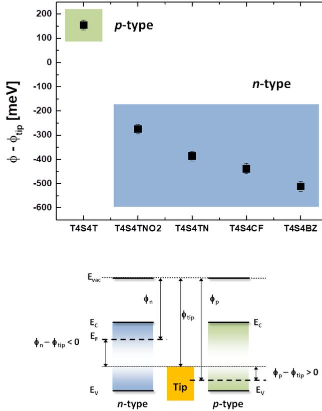
**Figure 10.** Surface electronic potential measured by KPFM for the fibers of **1-5** grown on glass and energy diagram for *p*-type and *n*-type charge carriers.
