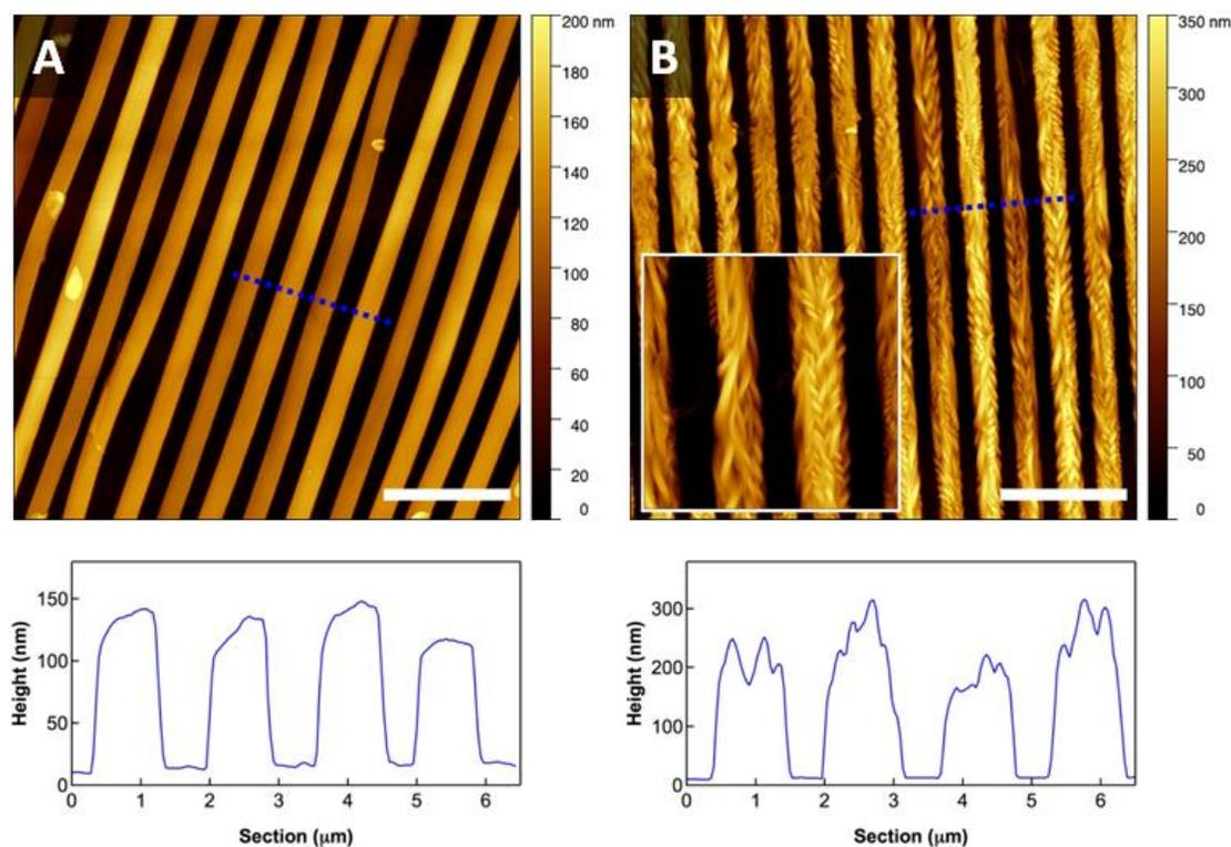
**Figure 2.** AFM images  $20 \times 20 \mu\text{m}^2$  and related height plots of the fibers of: (A) **2** (*T4S4TNO2*) and (B) **4** (*T4S4CF*) patterned according the Lithographically Controlled Wetting (LCW)<sup>21</sup> technique. Scale bars =  $5 \mu\text{m}$ . Inset image (B): zoom  $5 \times 5 \mu\text{m}^2$ .
