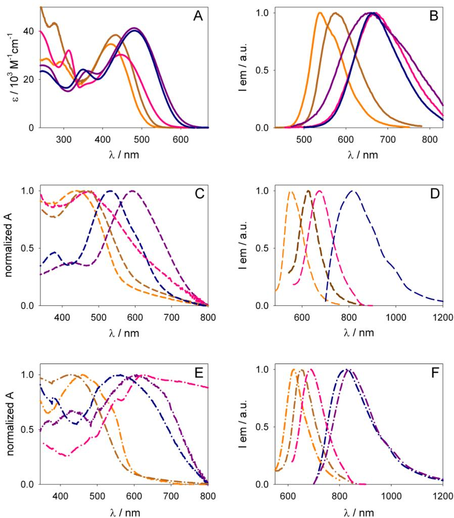
**Figure 3.** Absorption and emission spectra of **1** (*T4S4T*, yellow), **3** (*T4S4TN*, brown), **5** (*T4S4BZ*, pink), **4** (*T4S4CF*, blue) and **2** (*T4S4TNO2*, purple) in different conditions. A-B: air-equilibrated  $\text{CH}_2\text{Cl}_2$  at r.t.; C-D: drop-cast films on glass surfaces at r.t.; E-F: as crystalline fibers deposited on glass surfaces at r.t.
