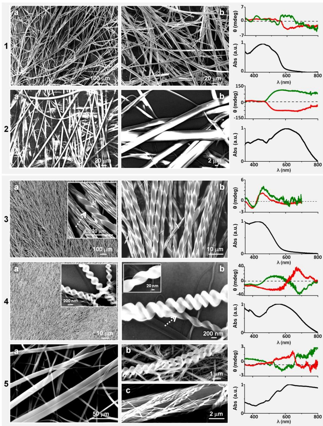
**Figure 1.** Scanning Electron Microscopy (SEM) images of fibers grown on glass from compounds **1-5** via the solvent-exchange method and Circular Dichroism plots of two different samples of the fibers of each compound.
