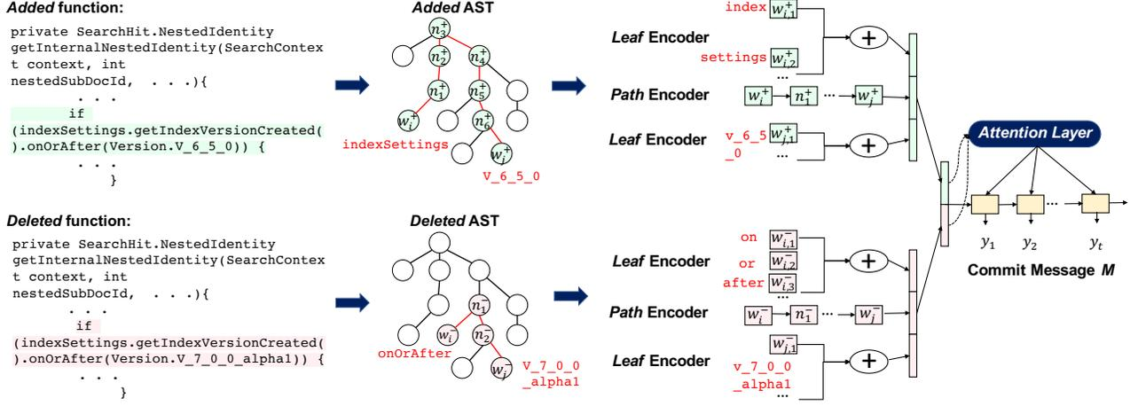
Fig. 6: Architecture of *AST2seq* with the example in Fig. 1, where *added* and *deleted* function denote the completed functions retrieved from the *diff*. The highlight path in *added* or *deleted* AST is one of paths extracted from tokens, e.g., *indexSettings*, *onOrAfter* in *diff* and  $n_i^{+/-}$  is the non-leaf node, e.g., “ForStmnt”, “Binary Expression”.
