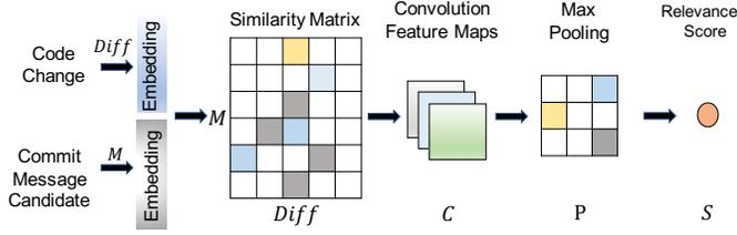
Fig. 7: Architecture of ConvNet.
