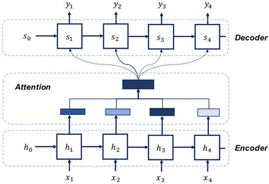
Fig. 3: An encoder-decoder model with an attention mechanism.
