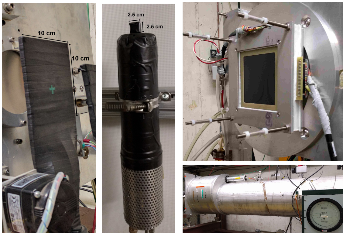
Figure 3. The FTBF instrumentation used for this beam test. The two left images show the scintillation counters: SC1 and SC4 respectively. The upper right image shows a Multi-Wire Proportional Chamber (MWPC) while the bottom right image shows a Cherenkov counter.
