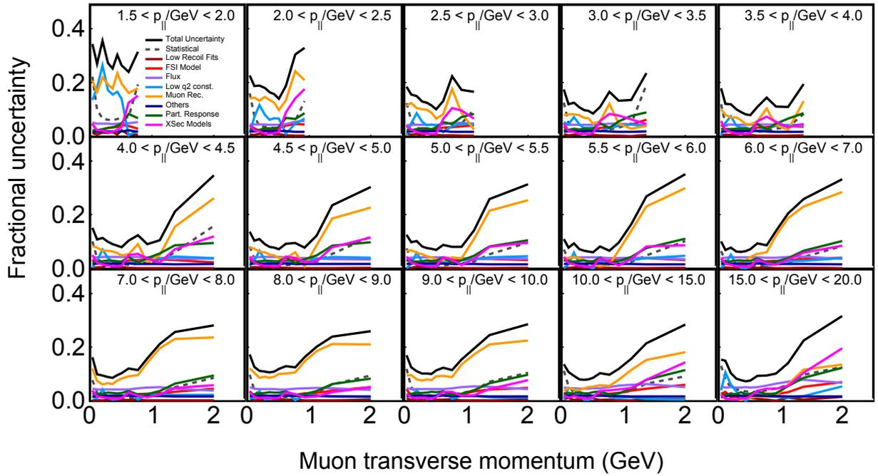
FIG. 3. Fractional systematic uncertainty on the double-differential cross section as a function of  $p_{\perp}$  and  $p_{\parallel}$ .
