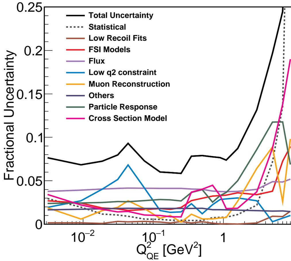
FIG. 4. Fractional systematic uncertainty on the single-differential cross section as a function of  $Q_{QE}^2$ .
