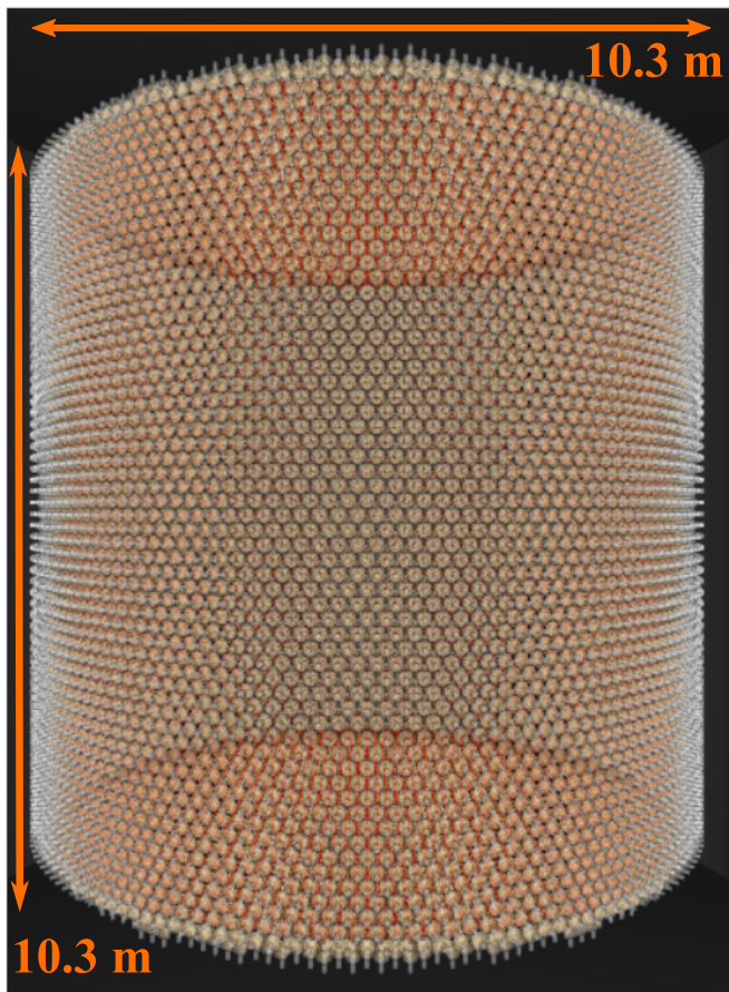
FIG. 23. A visualization of a 1-kT right cylinder active volume of LAB+PPO instrumented with 13,350 dichroicons produced by Chroma .
