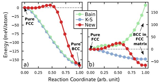
FIG. 3. Energy profile of the martensitic transformation. a) Transformation of an infinite iron single crystal from FCC (austenite) to BCC (martensite). b) Transformation of a plate of iron from FCC to BCC within the austenite matrix
