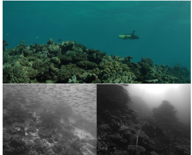
Fig. 1: Examples of challenges for AUV navigation in close-proximity to coral reef environments. (Top) A small AUV traversing at 1.0 m above a relatively flat coral reef. (Lower left) An image from the AUV showing cluttered and dynamic (fish) obstacles. (Lower right) An image showing strong lighting variations.
