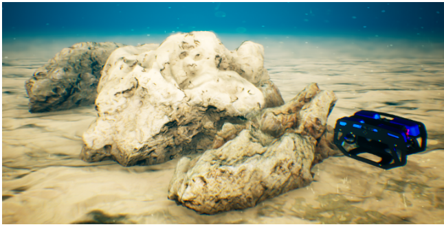
Fig. 7: An example 3D scene from the underwater simulator used for evaluating the probabilistic terrain mapping methodology. The robotic system is shown as a scale guide ( 0.5\text{m} \times 0.5\text{m} ) and is pointed in the direction of travel over the 3D structure.
