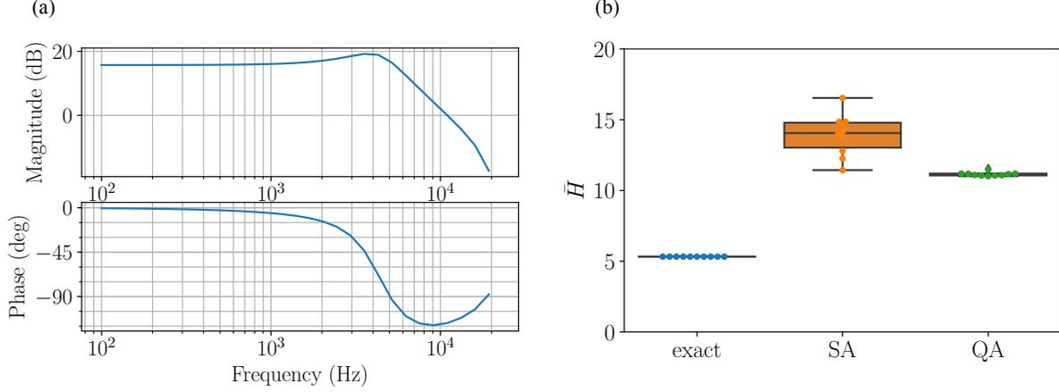
**Figure 2.** Result of dynamic audio quantization. (a) Bode plot of perception filter given in Eq. (22). (b) Value of evaluation function given in Eq. (27). The solution from the quantum annealing (green) is compared to that from the simulated annealing (orange) and exact solution (blue). The box-and-whisker plot is created by performing 10 numerical simulations.
