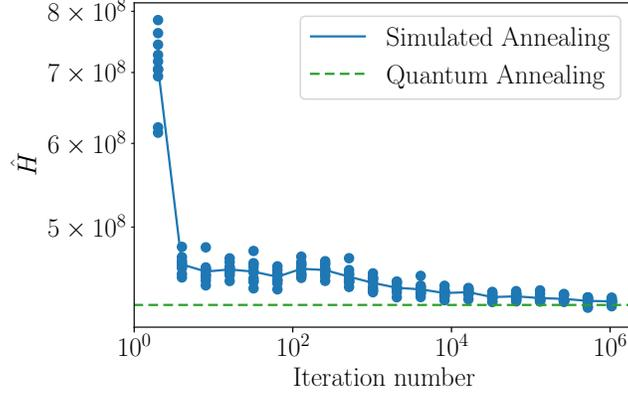
**Figure 3.** Iteration number for the simulated annealing versus the value of the evaluation function given in Eq. (15). At each value of iteration number, 10 computations are performed (blue dot) and the average value is plotted (blue solid line). The corresponding value of the evaluation function obtained with the quantum annealing method is also shown by the green dashed line.
