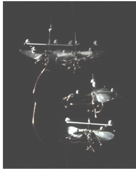
Fig. 13. Flight in which the robot takes off and hovers about a reference point in space with the help of feedback from a motion capture arena. The robot is subject to a small yaw bias torque that caused it to rotate leftward in this video [32].
