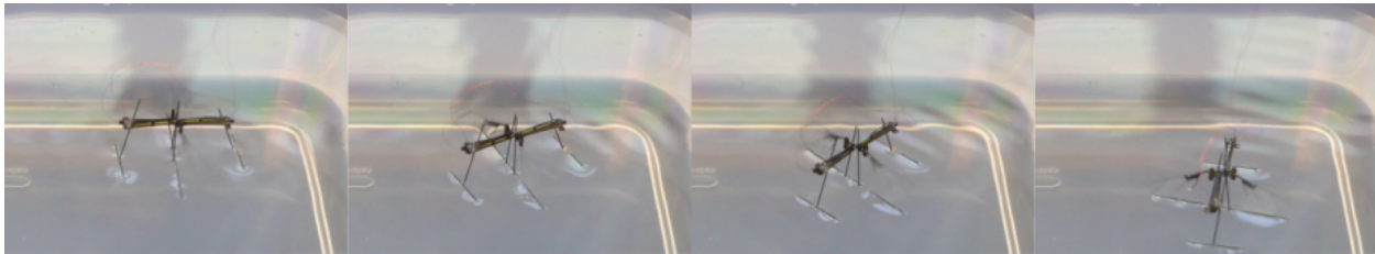
Fig. 20. Robot performing water surface locomotion and turning left with open loop control by flapping wings at 30 Hz, frames are captured at 0, 1, 2, and 3 s
