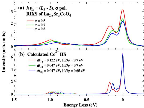
FIG. 4. Co  $L_3$ -edge RIXS spectra of  $\text{La}_{2-x}\text{Sr}_x\text{CoO}_4$  excited with  $\sigma$ -polarized x rays of energy 778 eV denoted by ( $L_3 - 3$ ). (a) RIXS spectra recorded at 20 K normalized to the incident beam intensity. (b) Calculated RIXS spectra for HS  $\text{Co}^{2+}$  of tetragonal symmetry with various parameter values for the tetragonal distortion  $\Delta t_{2g}$  and crystal field  $10Dq$ .
