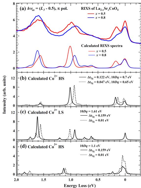
FIG. 5. (a) Measured Co  $L_3$ -edge RIXS spectra of  $\text{La}_{2-x}\text{Sr}_x\text{CoO}_4$  ( $x = 0.5$  and  $0.8$ ) with incident photon energy ( $L_3 - 0.5$ ) and  $\pi$  polarization. Calculated RIXS spectra for  $x = 0.5$  and  $0.8$  are obtained from the sum of the calculated RIXS spectra of (b) HS  $\text{Co}^{2+}$ , (c) LS  $\text{Co}^{3+}$ , and (d) HS  $\text{Co}^{3+}$  with estimated populations plotted in Fig. 6 (a). A spectral broadening has been applied to the summed spectra.
