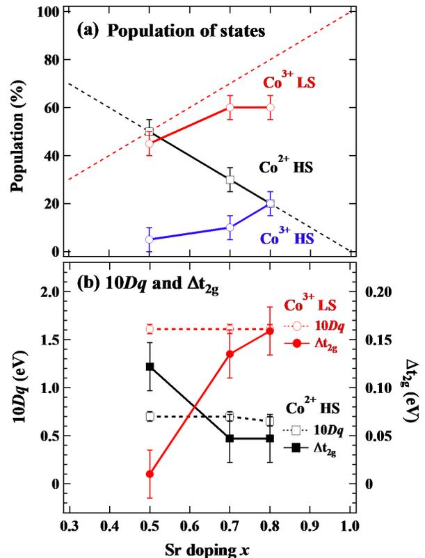
FIG. 6. Sr-doping dependence of (a) population of states estimated with RIXS results and (b) crystal field and tetragonal distortion of  $\text{CoO}_6$ . Black (red) broken lines in (a) are nominally expected  $\text{Co}^{2+}$  ( $\text{Co}^{3+}$ ) populations, respectively.
