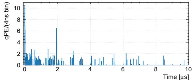
**Fig. 1** A typical trace from an approximately  $20\text{ keV}_{ee}$   $^{39}\text{Ar}$  event. The pulses from all PMTs are shown together.
