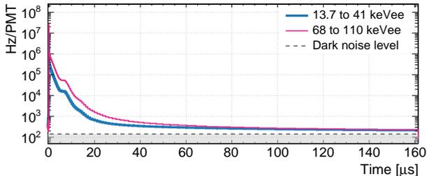
**Fig. 2** The average pulse shapes in different energy windows, normalized to the number of events in each histogram and to the total number of PMTs. Approximately 200 000 events were used for each energy window. The mean dark noise level of the PMTs is indicated by the dashed line. The pulse shapes do not reach the dark noise level even after 160  $\mu$ s due to an additional component of uncorrelated light as will be discussed in Sect. 4.
