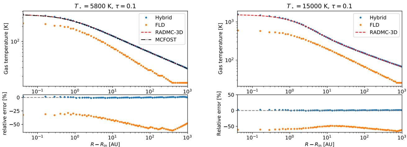
**Fig. 3.** Radial gas temperature profiles in the mid-plane of the disk following the test of Pascucci et al. (2004) for  $\tau = 0.1$ . We compare the gas temperature computed using MCFOST (black dotted-line) and RADMC-3D (red dashed-line), the hybrid method (M1+FLD, blue dots) and the FLD method alone (orange dots) in RAMSES. Left: central star temperature  $T_{\star,1} = 5800\text{K}$ ; right:  $T_{\star,2} = 15000\text{K}$ .
