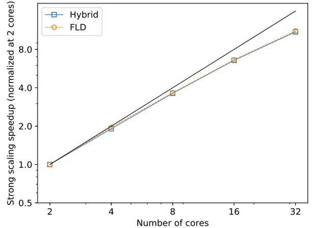
**Fig. B.1.** Strong scaling result for 2 to 32 cores in the test of Pascucci et al. (2004), with  $\tau = 100$ ,  $T_{\star} = 5800$  K. The ideal theoretical speedup is represented by the black line. We compare the strong scaling between the hybrid method (M1+FLD, blue squares) and the FLD method alone (orange circles). We normalize the speedup by that obtained with two cores.
