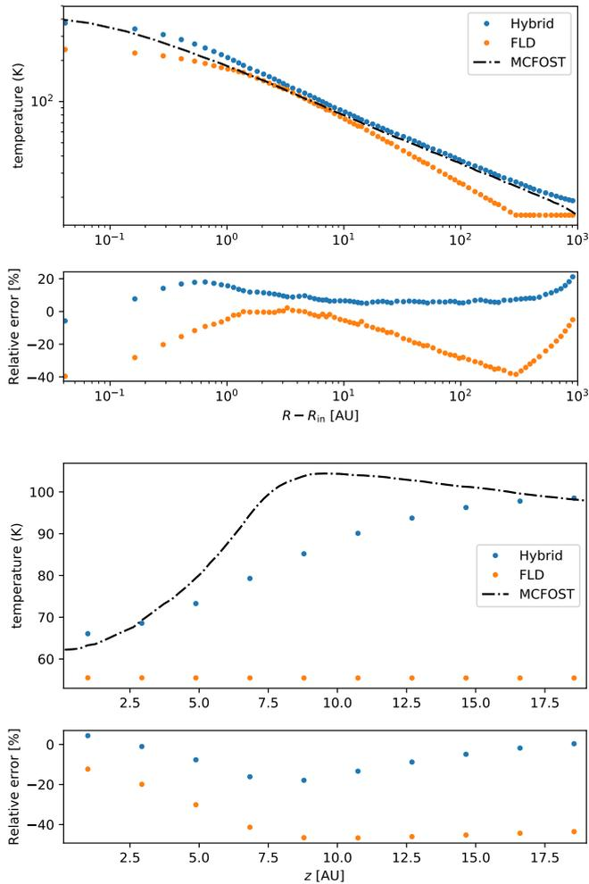
**Fig. A.1.** Gas temperature profiles, following the test of Pascucci et al. (2004). We compare the gas temperature computed using MCFOST, the hybrid method (M1+FLD) and the FLD method alone in RAMSES, with isotropic scattering.  $T_{\star} = 5800$  K and the integrated optical depth in the disk mid-plane is  $\tau = 100$ . Top: radial profile in the disk mid-plane. Bottom: vertical profile at a disk radius of 20 AU.
