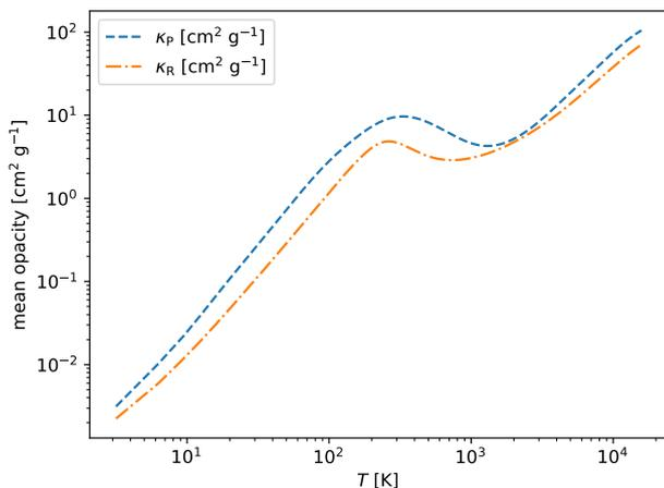
**Fig. 2.** Planck's (blue dashed curve) and Rosseland's (orange dot-dashed curve) mean opacities, as a function of temperature in the Pascucci setup.
