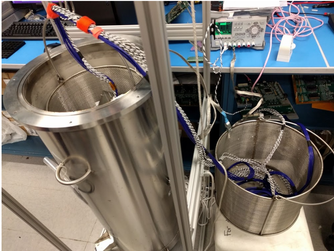
Figure 16: The FEMB production test stand, showing LN2 dewar, mesh bucket containing the CE Box inside the dewar, cold cables and WIB board. The code cables are held inside another wire mesh bucket outside the dewar during the test to minimize electronic noise pickup.
