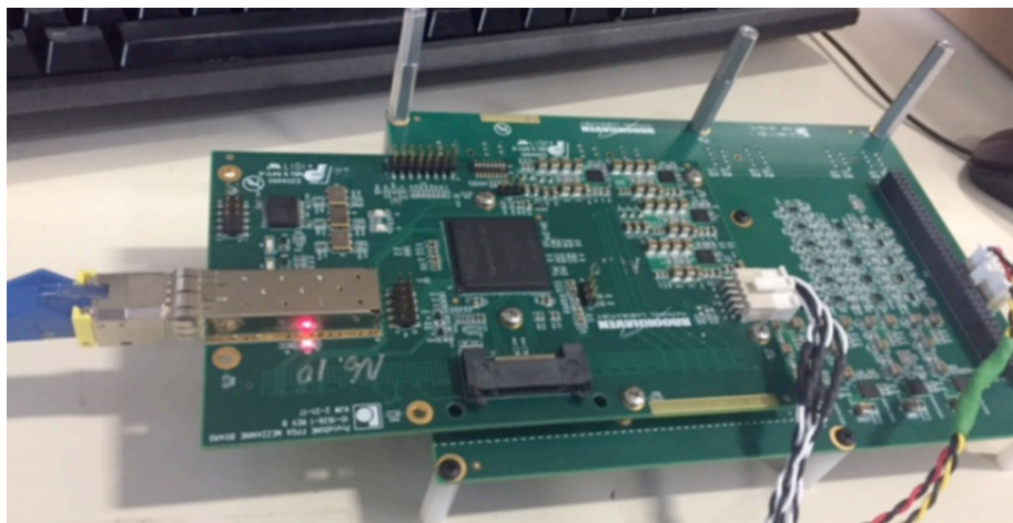
Figure 8: Quad-socket flash memory test board, controlled by an FEMB FPGA mezzanine with UDP Ethernet communication to the test PC.
