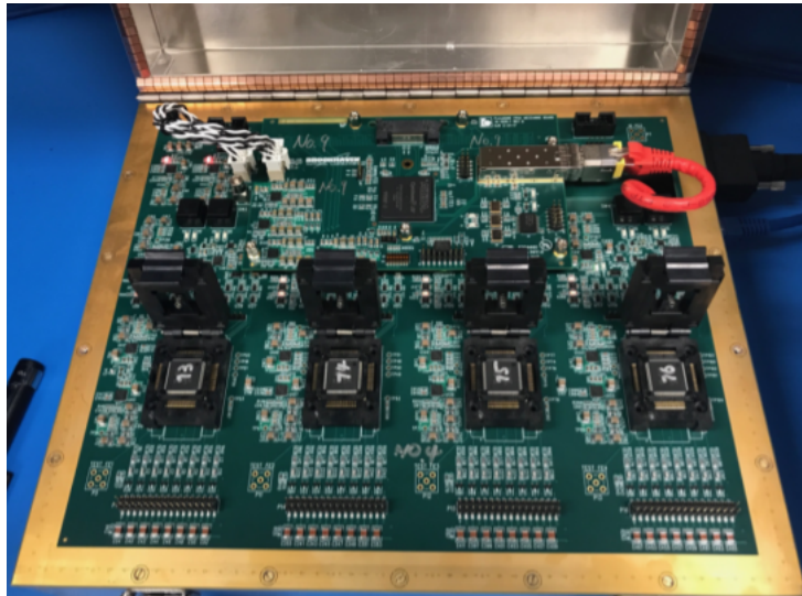
Figure 9: Quad-socket FE ASIC test board for room temperature tests. The test board is contained in a stainless steel box, which was closed by the test operator before initiating the test scripts to provide a Faraday cage during ASIC characterization.
