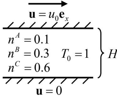
FIG. 6. Initial configuration of the thermal Couette flow.
