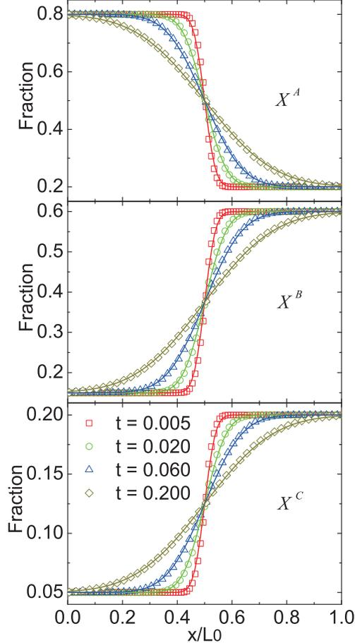
FIG. 4. Molar fractions in the diffusion process:  $X^A$  (top),  $X^B$  (middle), and  $X^C$  (bottom). Squares, circles, triangles, and diamonds denote DBM results at time constants  $t = 0.005$ ,  $0.02$ ,  $0.06$ , and  $0.2$ , respectively. Solid lines stand for the corresponding analytical solutions.
