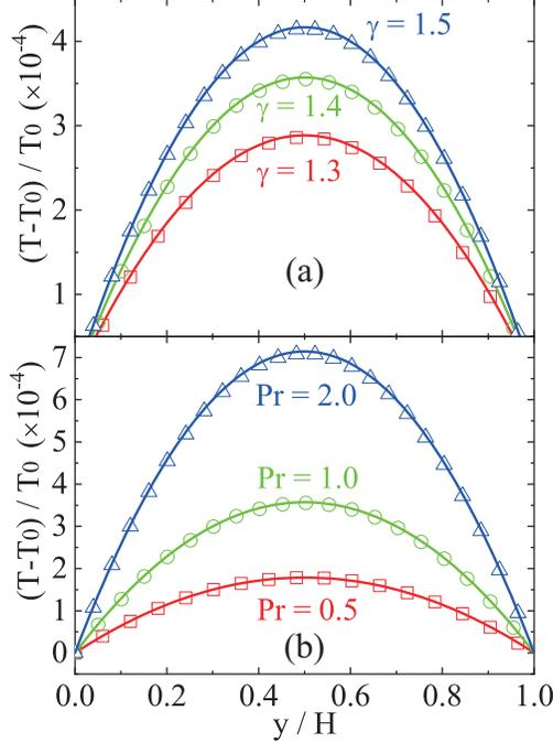
FIG. 8. Vertical distribution of the temperature in the steady Couette flow. (a) Cases with  $Pr = 1.0$  and  $\gamma = 1.3, 1.4$ , and  $1.5$ , respectively. (b) Cases with  $\gamma = 1.4$  and  $Pr = 0.5, 1.0$ , and  $2.0$ , respectively.
