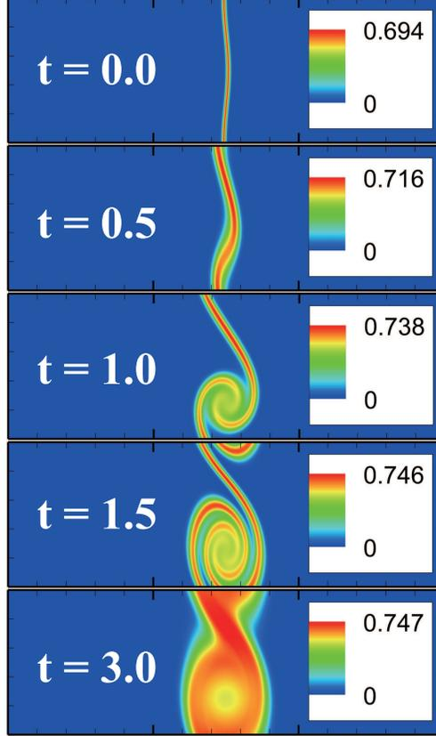
FIG. 13. Contours of the entropy of mixing at time constants  $t = 0.0, 0.5, 1.0, 1.5,$  and  $3.0$  in the evolution of KHI.
