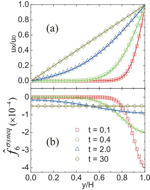
FIG. 7. Vertical distribution of the horizontal speed  $u_x$  (a) and nonequilibrium quantity  $\hat{f}_6^{Asneq}$  (b) in the thermal Couette flow. Squares, circles, triangles, and diamonds represent DBM results at time constants  $t = 0.1$ ,  $t = 0.4$ ,  $t = 2.0$ , and  $t = 30$ , respectively. Solid lines stand for the corresponding analytical solutions.
