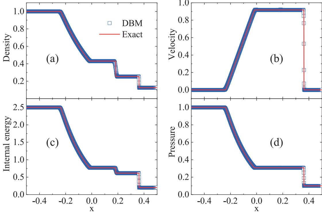
FIG. 11. Profiles of density (a), horizontal speed (b), temperature (c), and pressure (d) at a time constant  $t = 0.2$  in the Sod shock tube. Symbols represent DBM results, and solid lines stand for Riemann solutions.
