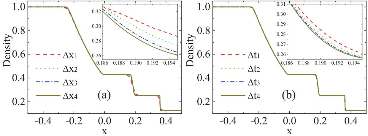
FIG. 10. Profiles of density at a time constant  $t = 0.2$  in the Sod shock tube with various spatial steps (a) and temporal steps (b).
