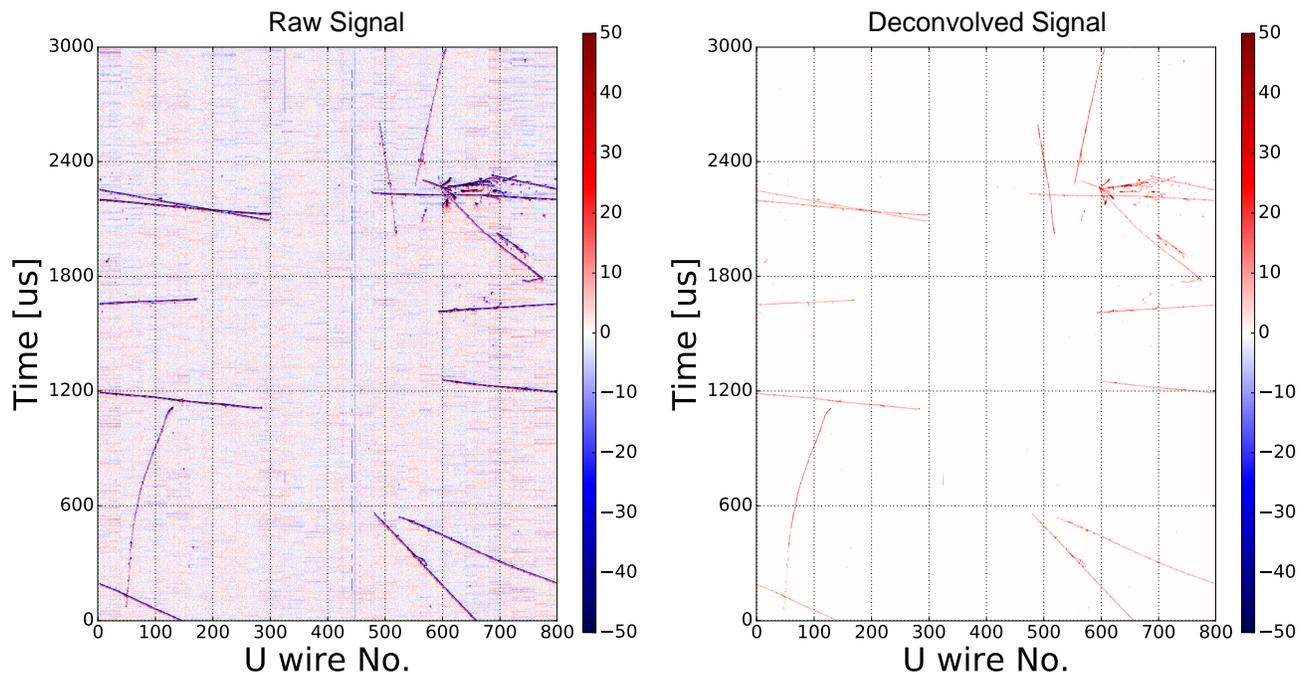
Figure 4.18: Comparison of raw (left) and deconvolved induction U-plane signals (right) before and after the signal processing procedure from a ProtoDUNE-SP event. The bipolar shape with red (blue) color representing positive (negative) signals is converted to the unipolar shape after the 2D deconvolution.
