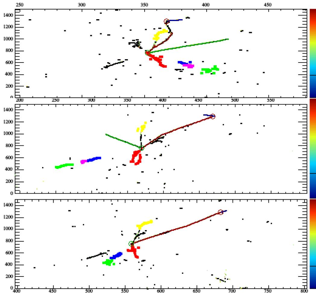
Figure 6.10: Event display for a well-classified  $n - \bar{n}$  signal event. The vertical axis is time ticks (each time tick corresponds to 500 ns), and the horizontal axis is wire number. The bottom view is induction plane one, middle is induction plane two, and the top is the collection plane. The color represents the charge deposited in each hit.
