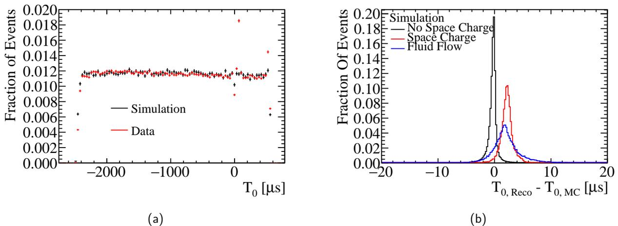
Figure 4.34: (a) The distribution of the reconstructed  $t_0$  for cosmic rays crossing the CPA in both data and MC. (b) the resolution on the reconstructed  $t_0$  in MC with different space charge effects applied; No space charge (black), space charge (red) and fluid flow (blue).
