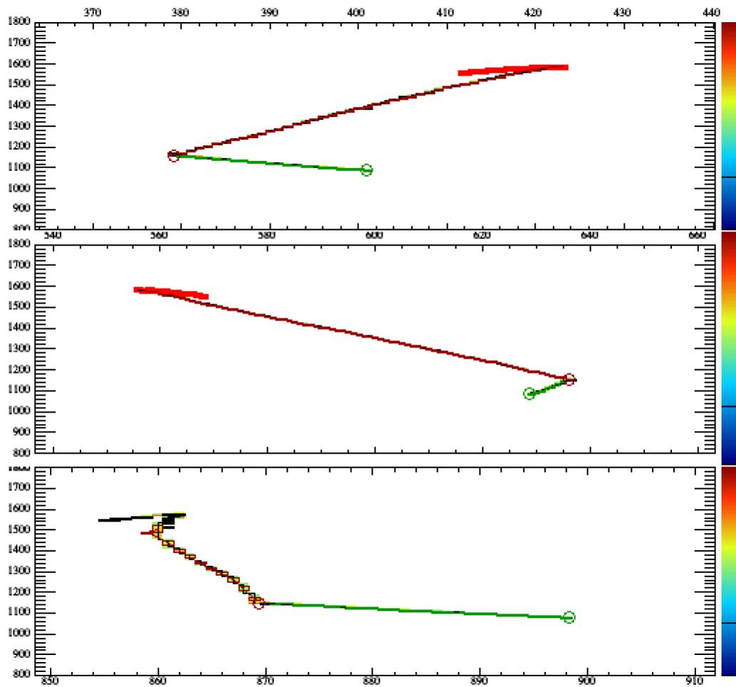
Figure 6.6: Event display for a well-classified  $p \rightarrow K^+ \bar{\nu}$  signal event. The vertical axis is time ticks (each time tick corresponds to 500 ns), and the horizontal axis is wire number. The bottom view is induction plane one, middle is induction plane two and top is the collection plane. The color represents the charge deposited in each hit.
