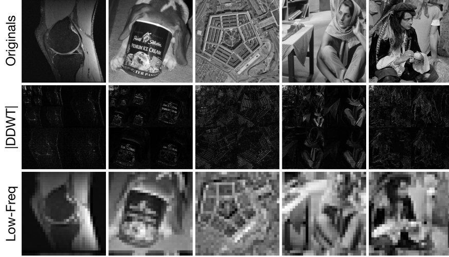
Figure 2: Wavelet Transforms of several different images. (Top) the original images, (Center) The magnitude of the Daubechies-4 wavelet transforms, (Bottom) the lowest-frequency bin of the wavelet transforms. Notably, the low frequency bin of the transform is not sparse (almost all values are non-zero).
