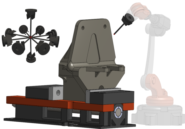
Figure 20: Support bracket setup with 5-axis milling and vise fixture. The highlighted components are used in accessibility analysis. The robot is abstracted by its DOF for orientation sampling.
