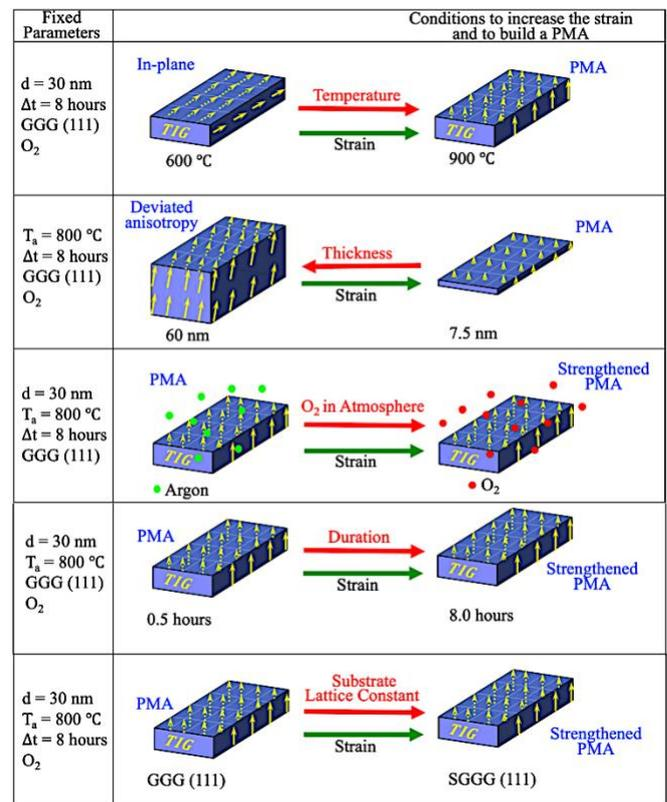
Fig. 6: Summary of how the annealing parameters, film's thickness and substrate's lattice constant build up or strengthen the PMA in sputtered TIG thin films. The left column shows a set of fixed parameters, while a variable parameter is analysed. The variable parameter is indicated by the red arrow. The green arrow indicates the increase of the strain, and thus, indicating the way to achieve higher PMA.
