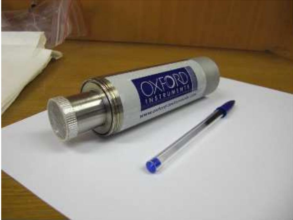
**Fig. 10.** Sealed single wire counter filled with TMAE vapors.
