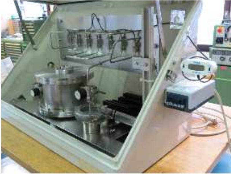
Fig. 19. Photograph of a setup for outgassing and filling with the gas of sealed gaseous detectors.
