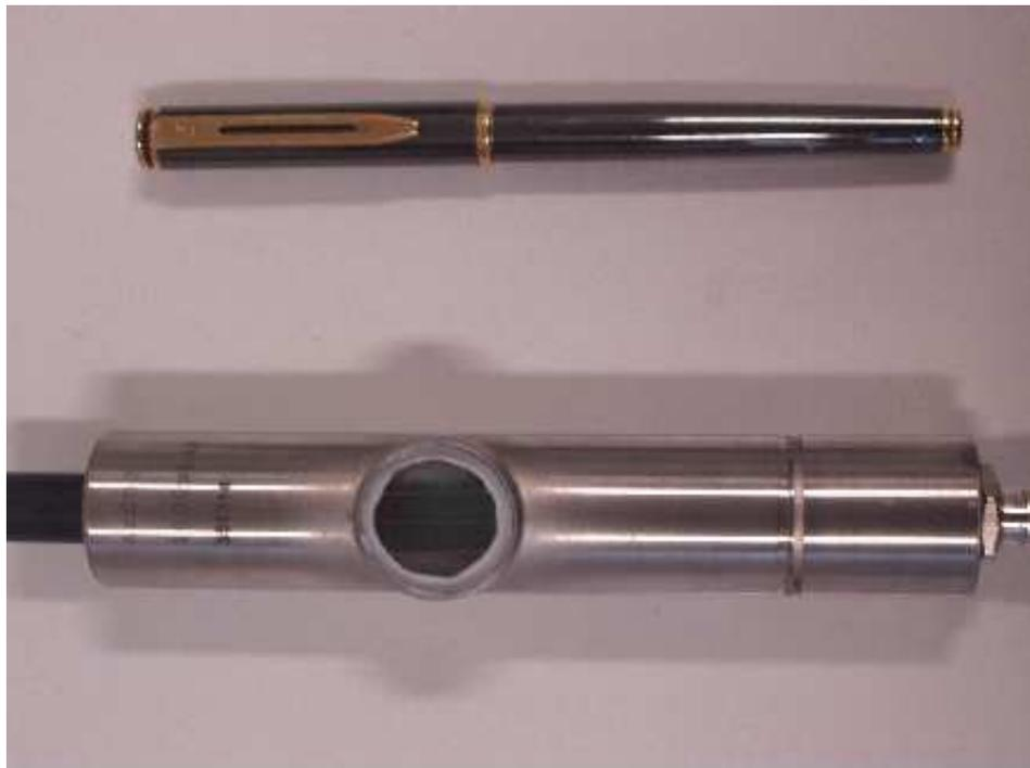
Fig. 2. Photo of the sealed gaseous detector with CsI photocathode developed in collaboration with Oxford Instruments Inc.
