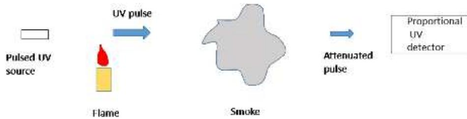
Fig. 31. Layout of the flame and smoke detector.
